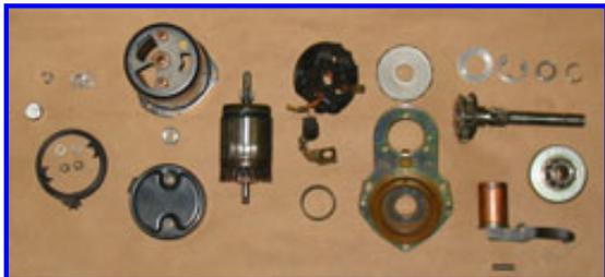
If you do a total disassembly of the starter, this is what you are likely to end up with (the solenoid body and nose casting are not shown here).
