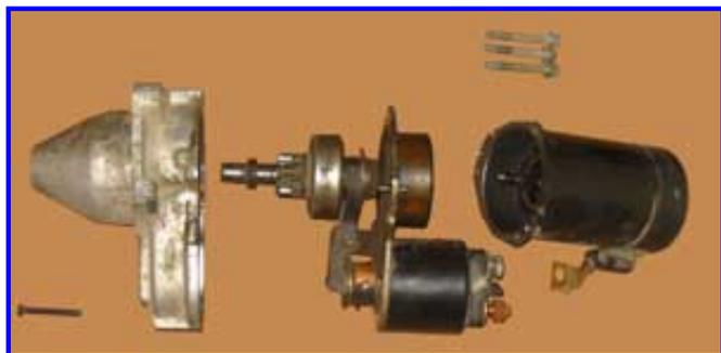
Remove the three bolts holding the motor housing to the nose casting, and remove the T20 bolt holding the solenoid to the casting. The nose casting can be pulled away, and the motor body can be pulled away as well, leaving three basic parts: the casting, the motor body, and the steel plate frame. Note: there are weak rivets also holding the motor housing to the plate, but pry them apart and discard them.
