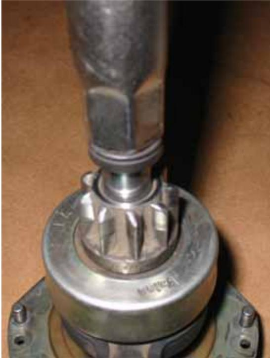
With a socket or equivalent, drive the outer ring down from its internal snap ring towards the pinion. In this picture I am using an item from a BMW toolkit to push it down.
