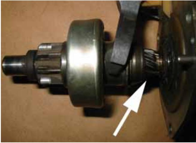
If you are just trying to stop a "run-on squeal" you may not need further disassembly. By cleaning out the curved splines between the pinion and the starter shaft, and cleaning the plunger you can restore free operation. Be sure to flush with plenty of solvent and blow dry with compressed air. You may want to lube with a VERY thin coat of a moly-based grease, such as CV joint grease.
